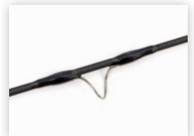
Flexible titanium single leg guides RECOIL Titanflex - made in USA. The first two guides under the tip have a serpentine design to reduce tangling of thin rigs.
